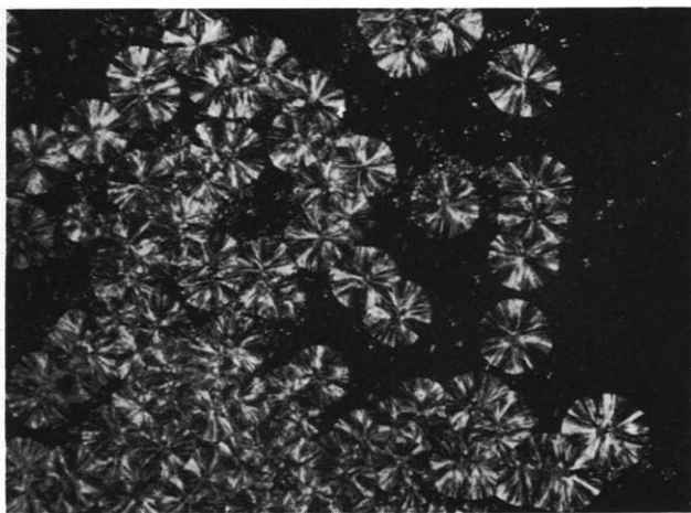
Figure 1 —Spherulites of transpolyisoprene crystallized at 50°C for 16 h. The large spherulites ( ca 130 \mu ) are the high melting form, the small spherulites ( ca 13 \mu ) are the low melting form
